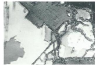
Fig. c: Two grains of quartz in a polished section of granodiorite. In this picture a grain boundary, (approximately down the middle) subgrain boundaries and cracks can be seen.
