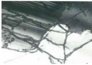
**Fig. b:** Two grains of quartz in a polished section of granodiorit. The marked contrast in the grain in the upper part of the picture reveals intracrystalline structure that is considerably harder to find by extinction contrast in transmitted polarised light microscopy.
