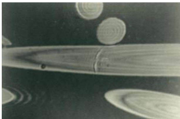
Fig. b: Glass fibres running vertically and obliquely to the surface. In the centre of the picture a crack in a glass fibre can be seen. Image width corresponds to 62,5 \mu\text{m}
