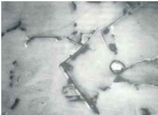
Fig. a: Polished cross section of an alloy with intermetallic deposits and impurities
