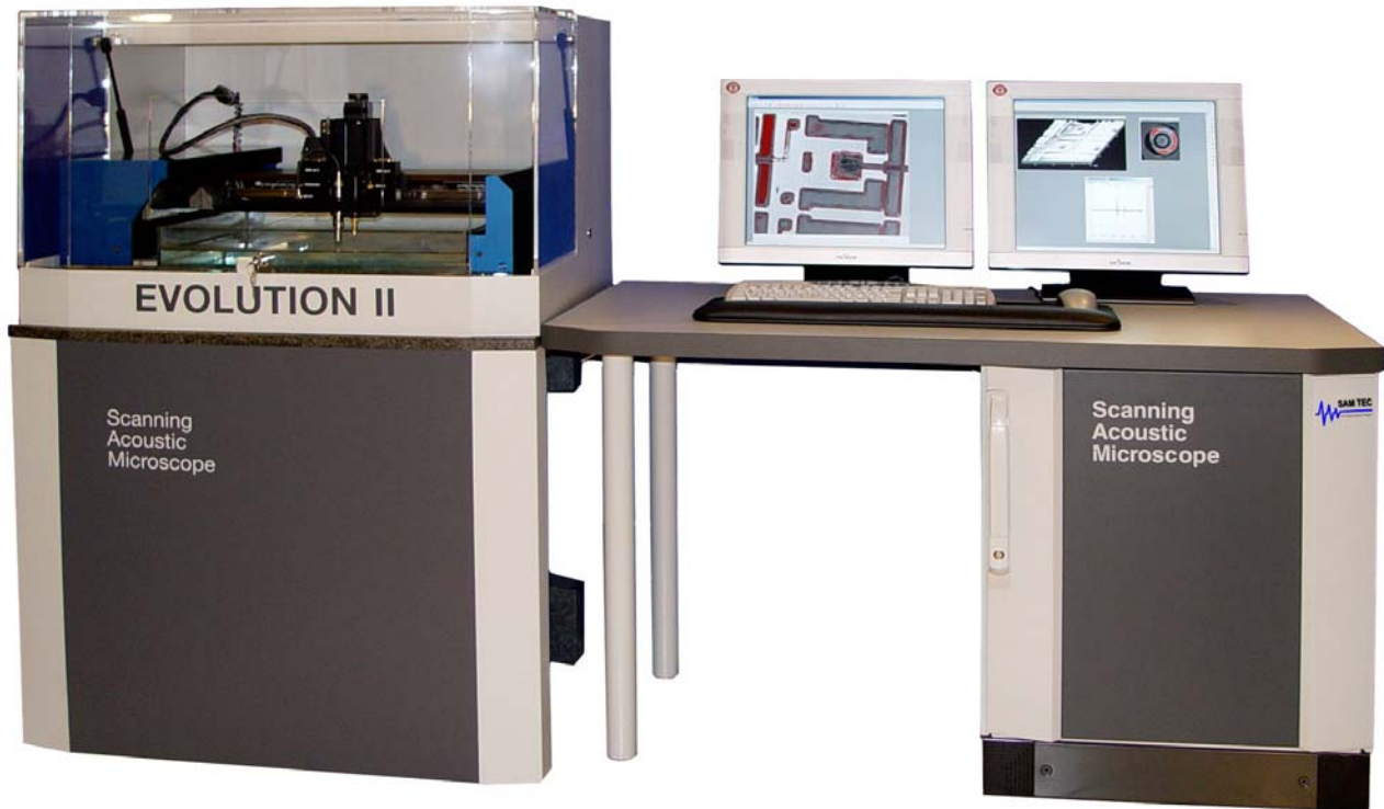
Fig. 1: Acoustic microscope Evolution II, working in the frequency range from 1 to 400 MHz. It consists out of a high speed high resolution linear scanner system, PC-controlled workstation, and various transducers. The customer can choose the set of transducers and the scanning system individually.
