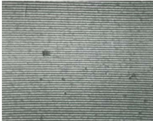
**Fig. 2:** Acoustic image of an optical grating used as a test of resolution. Distance between lines: 0,4  $\mu\text{m}$ , Frequency: 2 GHz, 2000x
