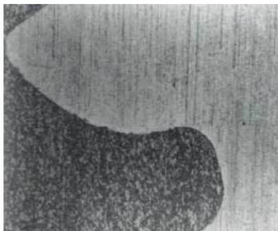
Fig. b: On this part of the gear wheel scratches can be seen which were probably caused during aftertreatment of the surface.
