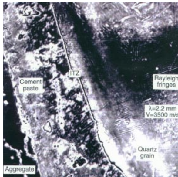
Fig. 1: Granitic aggregates without silica fume Frequency: 800 MHz Size: 312 \times 312\ \mu\text{m}
